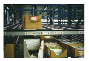
The second form is put to light. This process is primarily used to support batch picking. After the items are batch picked, they are brought to a put to light area. Each location represents an order. When an item is scanned, a lighted display at each location presents the quantity to put in the location.
